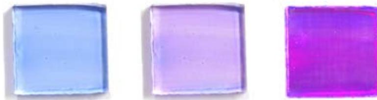
**Figure 1:** From left to right, photographs of a Rz-coated clear BioClean™ glass sample: (i) before UV irradiation, (ii) after 20 min UV irradiation and (iii) as in (ii) but under low UV light illumination in order to reveal the highly fluorescent nature (photographed here) of the photocatalytically generated Rf.
