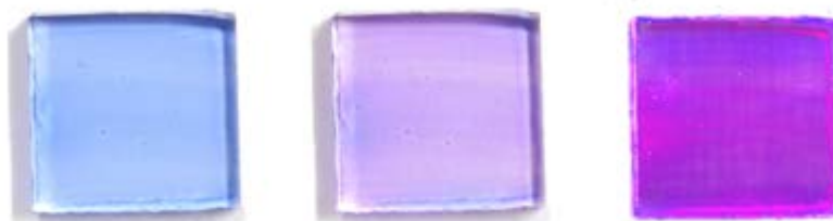
Figure 1: From left to right, photographs of a Rz-coated clear BioClean™ glass sample: (i) before UV irradiation, (ii) after 20 min UV irradiation and (iii) as in (ii) but under low UV light illumination in order to reveal the highly fluorescent nature (photographed here) of the photocatalytically generated Rf.
