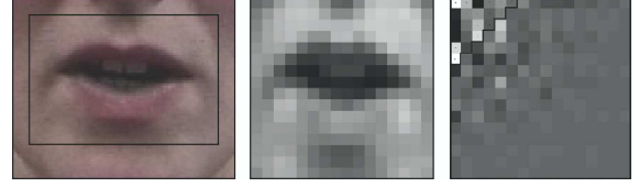
Fig. 2. Feature extraction from left to right: mouth ROI cropping, sub-sampling Y channel to 16 by 16 pixels, 2D DCT coefficients showing 5 by 5 triangular mask.
