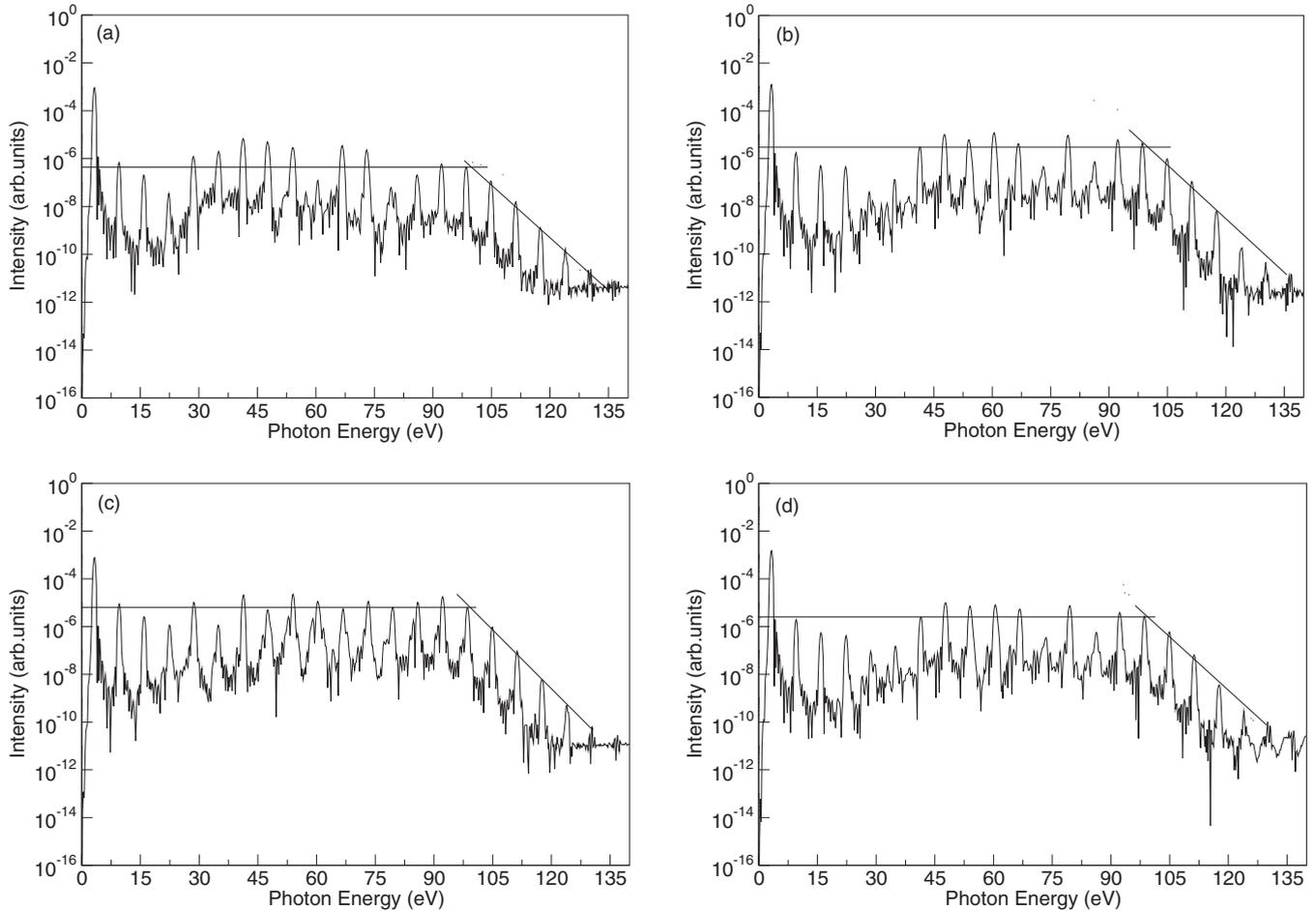
FIG. 3. The harmonic spectra obtained for  $\text{Ne}^+$  irradiated by 390 nm laser pulse, as obtained through the dipole length operator, at peak intensity of  $10^{15} \text{ W cm}^{-2}$ . The spectra are obtained when the following  $2s^2 2p^4$  thresholds are retained: (a)  $^3P^e$  and  $^1S^e$ , (b)  $^3P^e$  and  $^1D^e$ , (c)  $^1S^e$  and  $^1D^e$  thresholds, and (d) all three thresholds.
