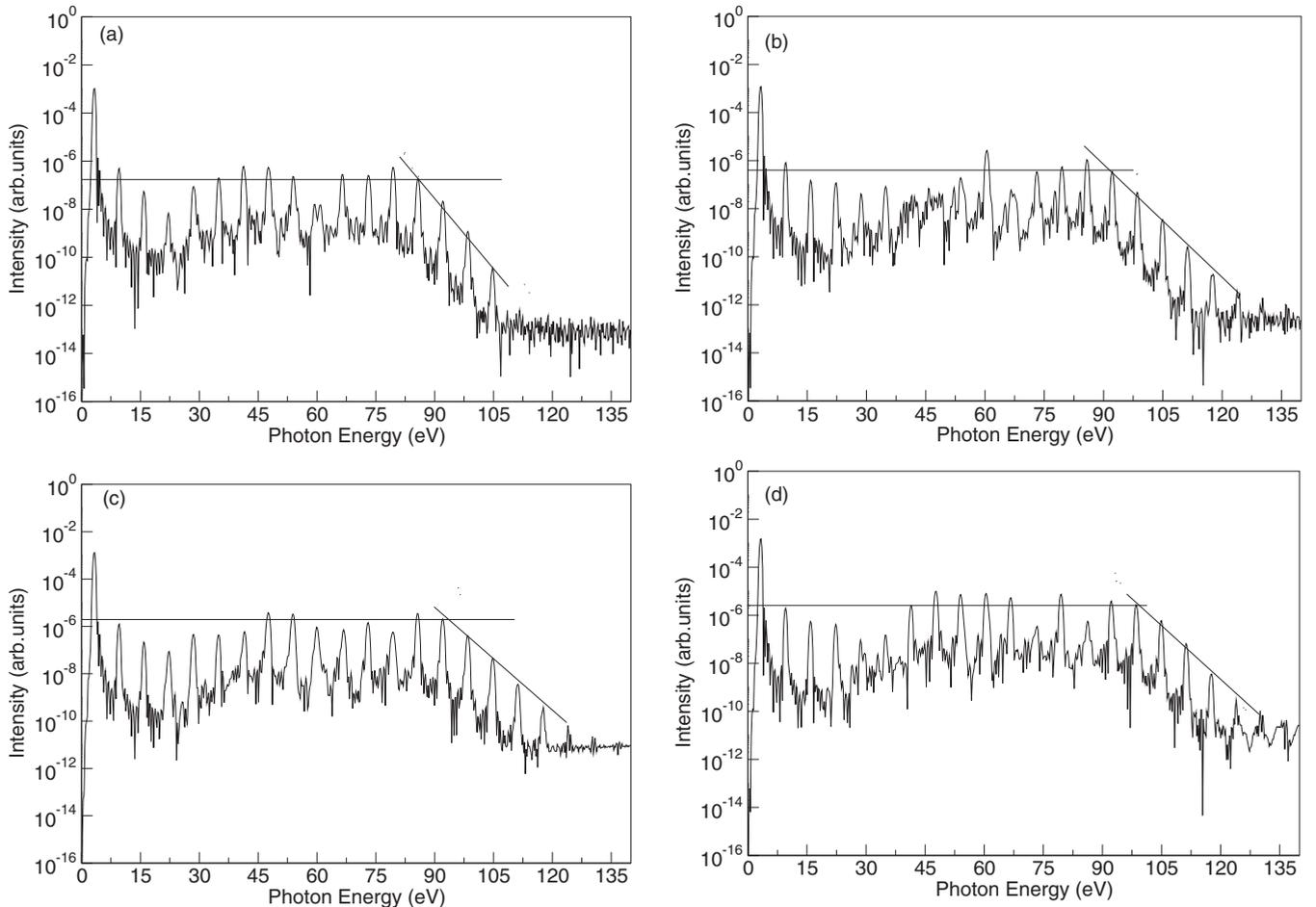
FIG. 1. The harmonic spectrum obtained by 390 nm laser pulse with a total duration of 10 cycles generated from  $\text{Ne}^+$  calculated from the dipole length, at different laser peak intensities: (a)  $7 \times 10^{14} \text{ W cm}^{-2}$ , (b)  $8 \times 10^{14} \text{ W cm}^{-2}$ , (c)  $9 \times 10^{14} \text{ W cm}^{-2}$ , and (d)  $10^{15} \text{ W cm}^{-2}$ .
