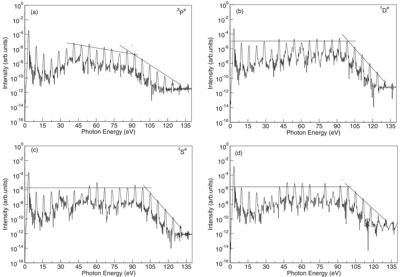
FIG. 2. Harmonic spectra for  $\text{Ne}^+$  irradiated by 390 nm laser pulse as calculated through the dipole operator, at peak intensity of  $10^{15} \text{ W cm}^{-2}$ . The  $\text{Ne}^{2+} 2s^2 2p^4$  residual-ion states retained are (a)  $^3P^e$ , (b)  $^1D^e$ , (c)  $^1S^e$ , and (d) all three states.
