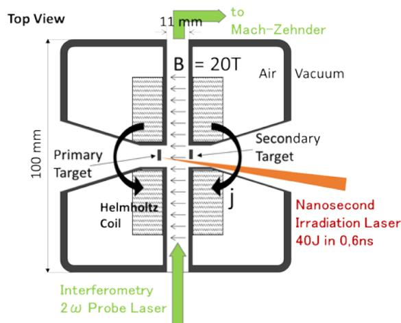
**Fig. 1 :** Top view of the experimental setup. Two targets (primary and secondary targets) look at each other. Their normal is parallel to the magnetic field lines generated by the Helmholtz coil. A longitudinal aperture allows the laser to irradiate the primary target. A radial aperture allows a clear line of sight to the plasma
